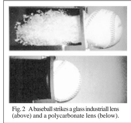
Fig. 2 A baseball strikes a glass industrial lens (above) and a polycarbonate lens (below).
